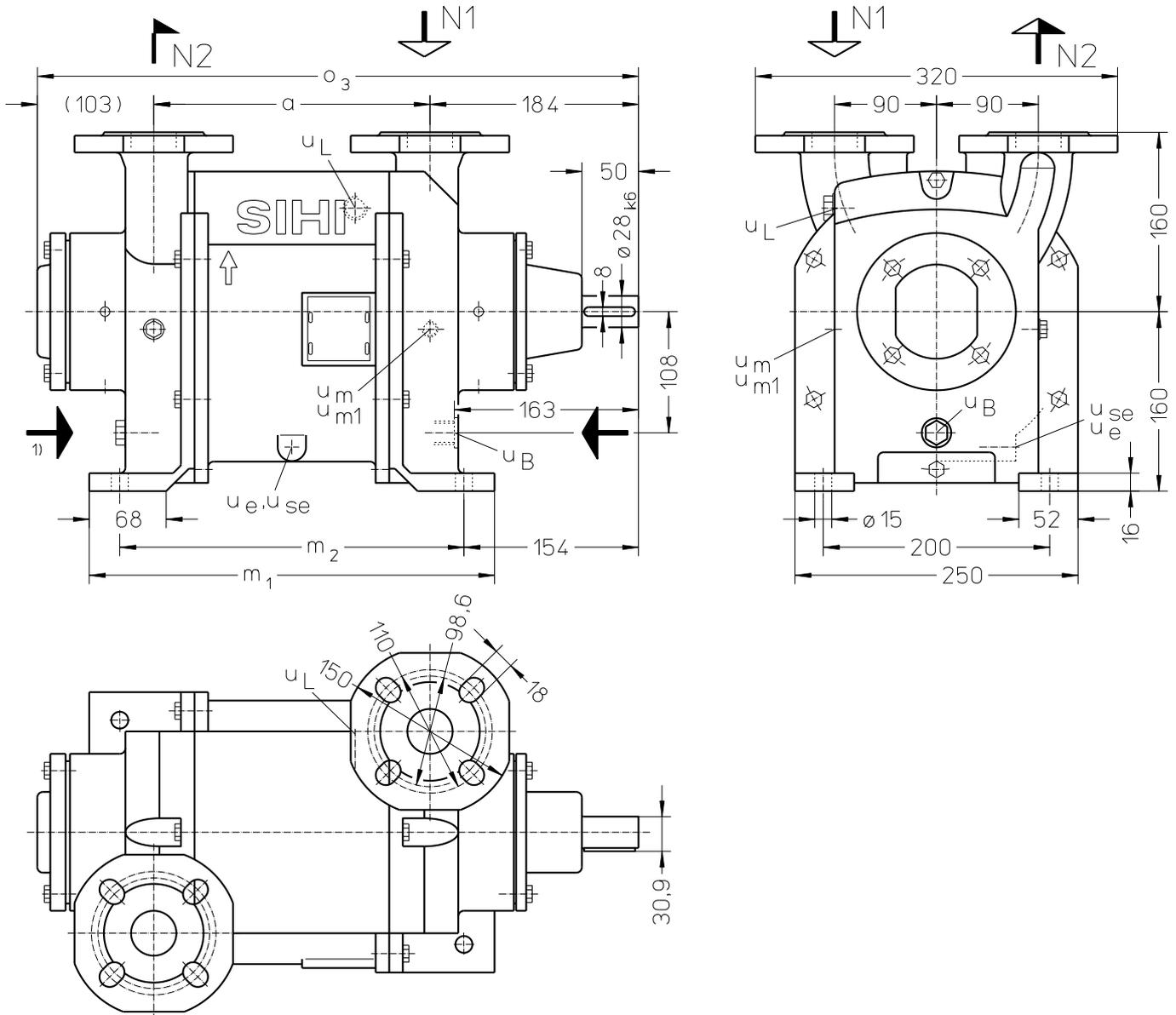
1) = Connection  $u_B$  on both sides is only necessary for LPH 40516
