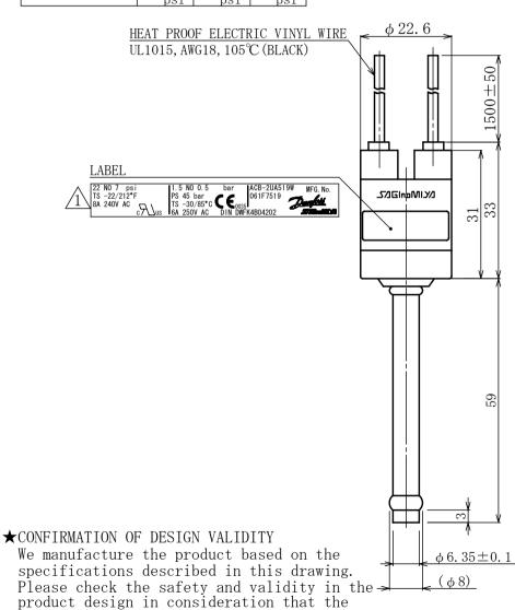
AT BRAZING OF PIPES, WRAP THE SWITCH BODY WITH WET CLOTH AND KEEP THE TEMPERATURE OF SWITCH BODY UNDER 100°C
