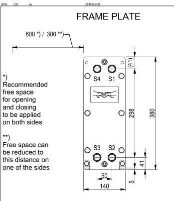
Space between pressure plate and supporting column should be kept free from fixed installations!
