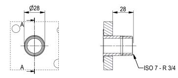
All dimensions in millimeters (mm)
