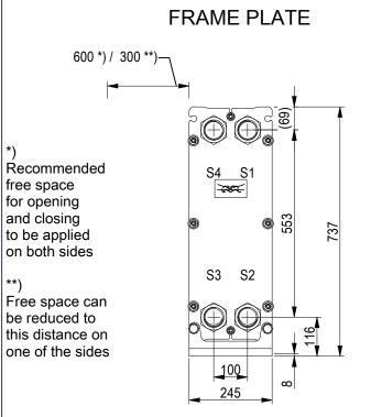
Space between pressure plate and supporting column should be kept free from fixed installations!
