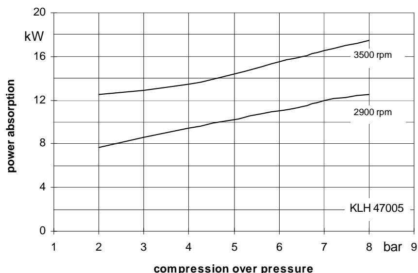
The values indicated for volume and power absorption are valid for compression of dry air at 20°C from atmospheric pressure (1013 mbar) of the respective compression pressure with water at 20°C as service liquid. Tolerance of the curve values is 10%. The compression pressure in bar is indicated as pressure above the atmospheric pressure.
