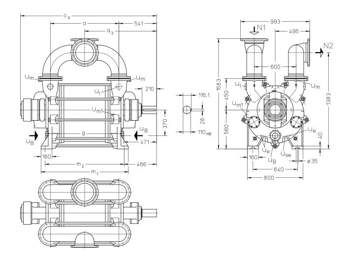
N 1 = gas inlet DN 250 N 2 = gas outlet DN 250
