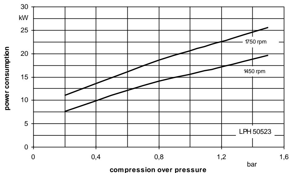
The suction volume and power consumed values are valid for compressing dry air at 20°C at atmospheric pressure (1013 mbar) to the corresponding overpressure using water as the service liquid with a temperature of 20°C. The curve tolerance is 10%. The compression pressure is expressed in bar relative to ambient air pressure.
