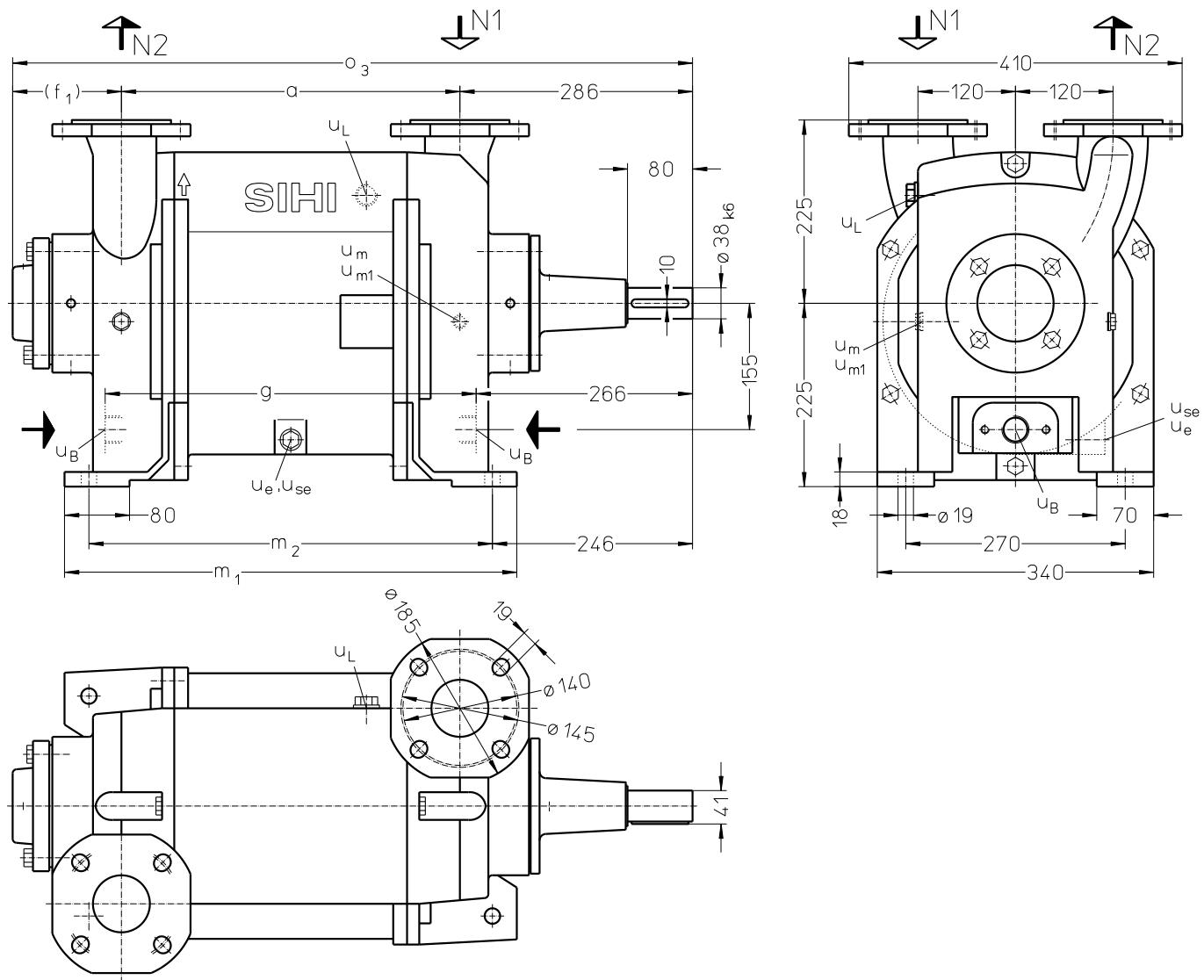
N 1 = Gas inlet DN 65 (according to DIN EN 1092 PN 10, 4 bolt)
